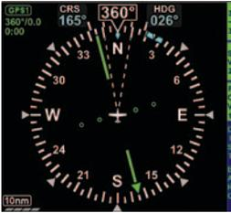
Figure 3-13 Narrow Horizontal FOV
