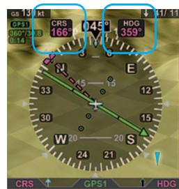
Figure 3-5 CRS and HDG display
