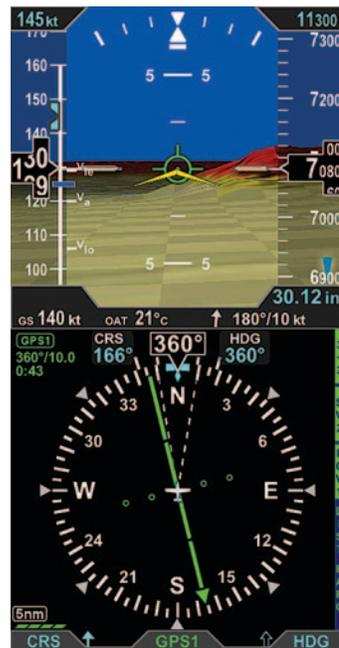
Figure 4-1 Terrain Warning System Alerts
