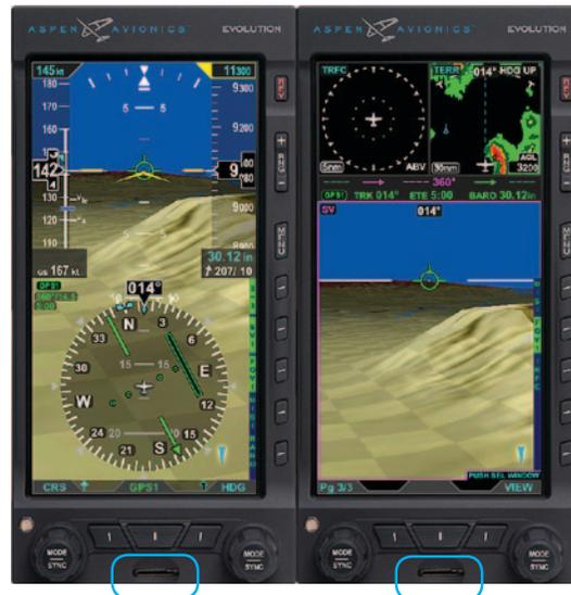
Figure 8-3 microSD Card Slot Locations
