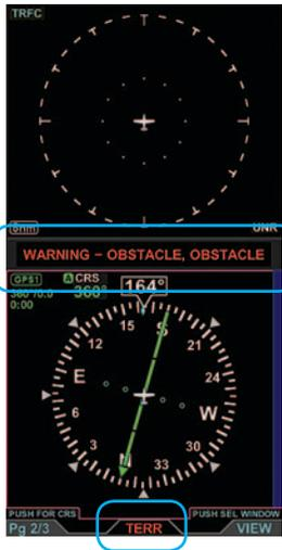
Figure 4-13 MFD Obstacle WARNING, Synthetic Vision Not Selected
