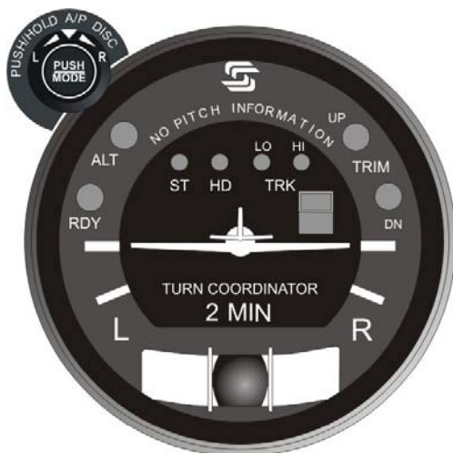
Fig. 2-4. AP Display, Turn Coordinator Failure (System Twenty)
