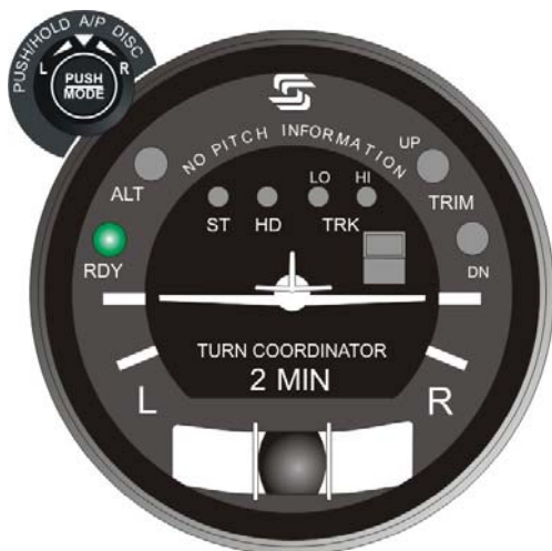
Fig. 2-3. AP Display, RDY for Operation (System Twenty)
