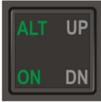
Fig. 2-28. ALT HOLD ON/OFF Switch Display, ALT HOLD Mode Engaged (System Thirty ALT)
