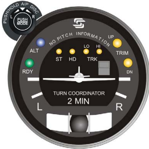
Fig. 2-6. AP Display, RDY, ALT, ST, HD, LO TRK, HI TRK, TRIM UP, TRIM DN Lamps Illuminated at Power-Up (System Thirty)
