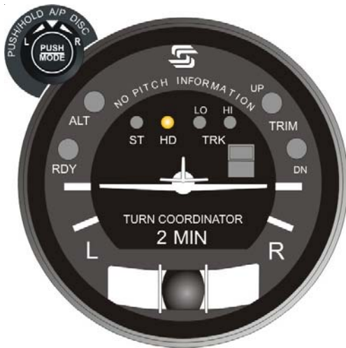
Fig. 3-2. AP Display, HD Mode Engaged
