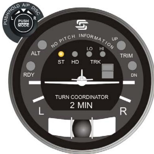
Fig. 2-17. AP Display, ST Mode Engaged (System Twenty)
