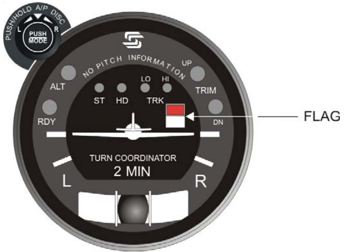
Fig. 2-5. AP Display, Low Voltage Flag (System Twenty)
