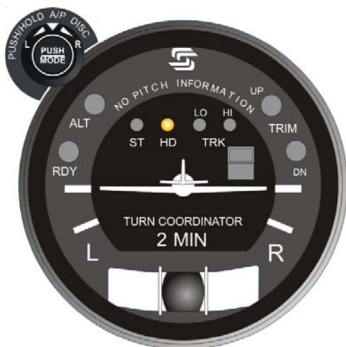
Fig. 2-22. AP Display, HD Mode Engaged (System Thirty)
