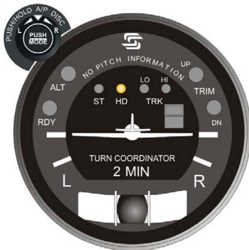
Fig. 2-18. AP Display, HD Mode Engaged (System Twenty)
