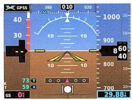
When GPSS is selected on the G5, GPSS turn commands are converted into a heading error signal to the autopilot. When the autopilot is operated in HDG mode, the autopilot will fly the turn commands from the GPS navigator. If the GPSS data is invalid (for example, if there is no active GPS leg) or the selected HSI source on the G5 HSI is not GPS, the annunciated GPSS text will be yellow and a zero turn command will be sent to the autopilot.
